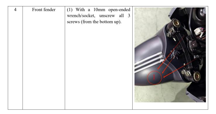
3.1.2 (1) Disassembly and replacement sequence of front cover of frame
